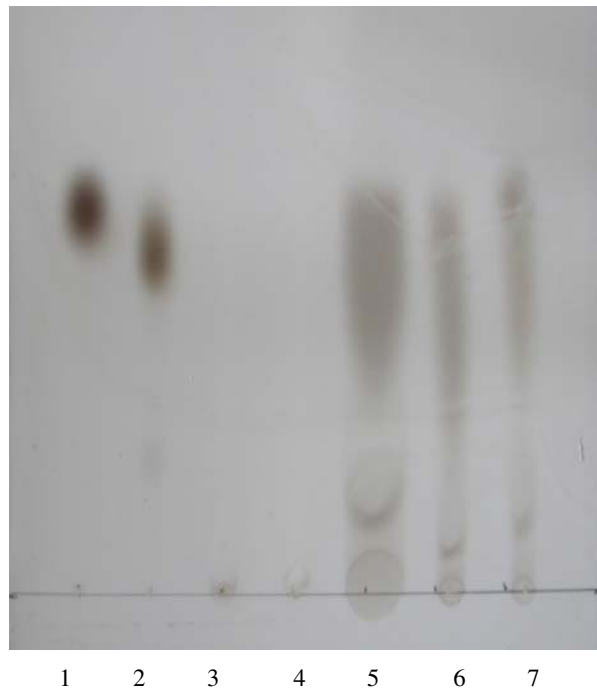
Fig. 5 Thin-layer chromatogram (TLC) of the end products of starch after hydrolysis with the crude amylase from the yeast strain A11. Lane 1 glucose, lane 2 maltose, lane 3 unhydrolyzed soluble starch, lane 4 unhydrolyzed cassava starch, lane 5 hydrolyzed soluble starch, lane 6 hydrolyzed cassava starch, lane 7 hydrolyzed cassava starch. The end products of starch hydrolysis was analyzed by using TLC plate (Silica gel 60, MERCK, Germany) with the solvent system n -butanol–pyridine–water (6:4:3) and a detection reagent comprising 2.0% diphenylamine in acetone–2.0% aniline in acetone–85.0% phosphoric acid (5:5:1 by volume)
